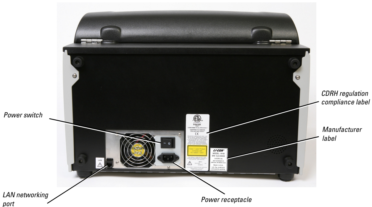
Figure 2-3. Closeup of the Odyssey ® CLx rear panel showing the power receptacle and LAN port (use only the supplied networking cable). Also shown are the CDRH regulation compliance label, the manufacturer label and the power switch. The power switch can be left in the 'on' position.
